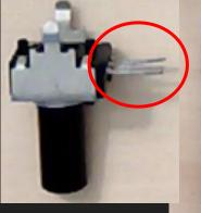
Insert the 10k Potentiometer into rows 14, 15, and 16 column a, facing outward to the left.
